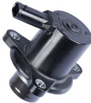
Following a load change in a charged engine, turbo bypass valves keep the number of rotations in the turbocharger constant, thus assuring that sufficient power is immediately available for acceleration. The 6<sup>th</sup> generation of solenoid valves just ordered – Pierburg’s Turbo Bypass Valve Gen. 6 – is characterized by especially short opening times, as well as low weight and small size.
