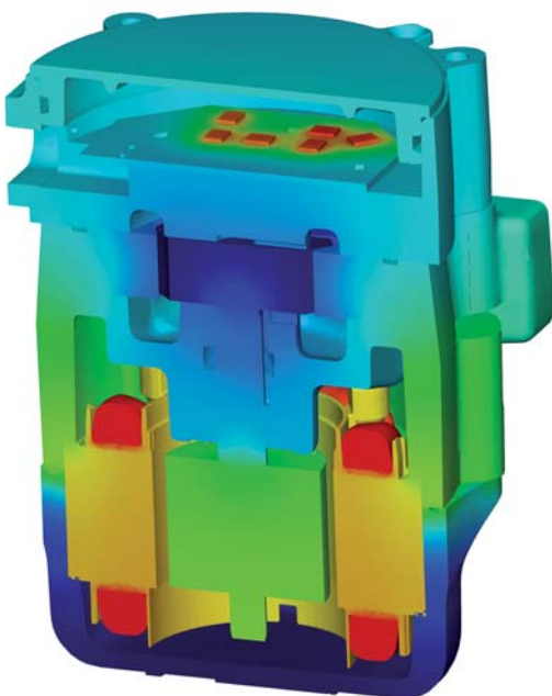
④ CFD analysis of an electric powered oil pump: typical temperature distribution
