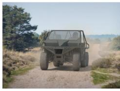
range of more than 1,000 kilometres and a top speed of 90 km/h are possible, depending on the vehicle's configuration. Up to four Ermine vehicles can be transported by cargo helicopters such as the CH-47 or CH-53.
