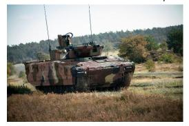
modules in numerous variants. This allows each basic vehicle to be configured, for example, as an infantry fighting vehicle, air defence system, command vehicle or medical vehicle. The mission module can be changed between variants throughout the life of the platform. By making the drive module identical, this system significantly reduces lifecycle costs and also allows military users to adapt force structures or develop new capabilities in a short time to react to changes on the battlefield.
