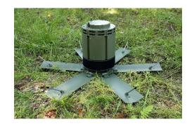
The ADW's effector is a SMArt 155 sensor-fuse sub-munition that attacks targets from above where their armour protection is weakest. This way, it can successfully engage even heavily armoured vehicles within a radius of over 100 metres.
