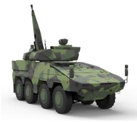
per minute. Featuring an extensive elevation range of -10 to +85 degrees, it can reliably engage small and swarm targets at distances of up to 3,000 metres. The turret holds 252 rounds of ammunition, ready to fire. As an option, the Skyranger 30 turret can also be equipped with two SHORAD surface-to-air missiles, doubling the system's engagement range to 6,000 metres.
