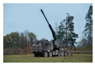
future growth potential. The L60 can project low-cost standard projectiles (boattail; base bleed; V-LAP) more than 80 kilometres. Precision guided munitions such as the Vulcano will allow to engage high-value targets at even greater ranges.
