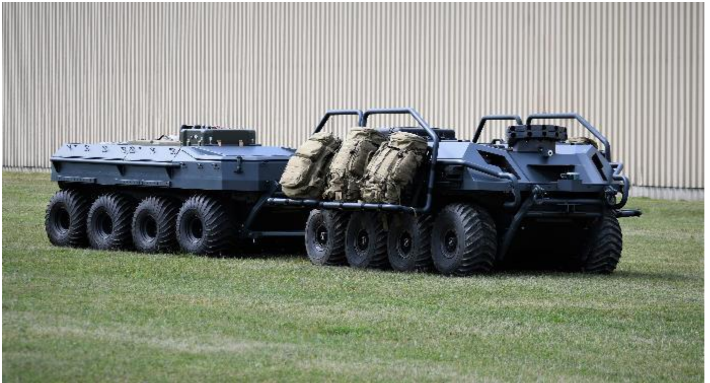
Rheinmetall Mission Master – Cargo equipped with its new trailer
